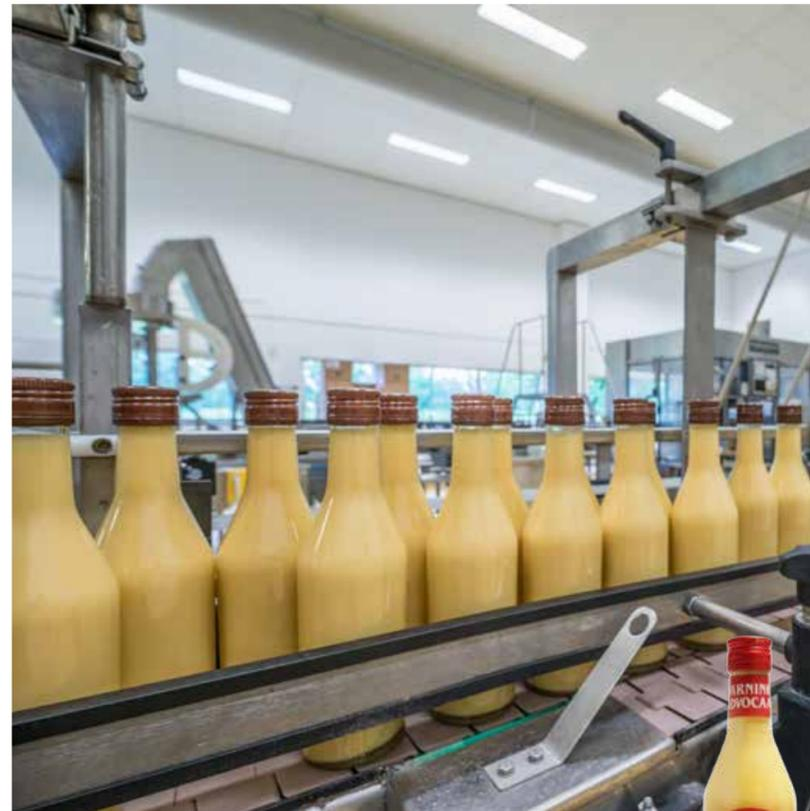
The bottling plant at Middelharnis can process 6-7000 bottles per hour, including cleaning, filling and labeling.
