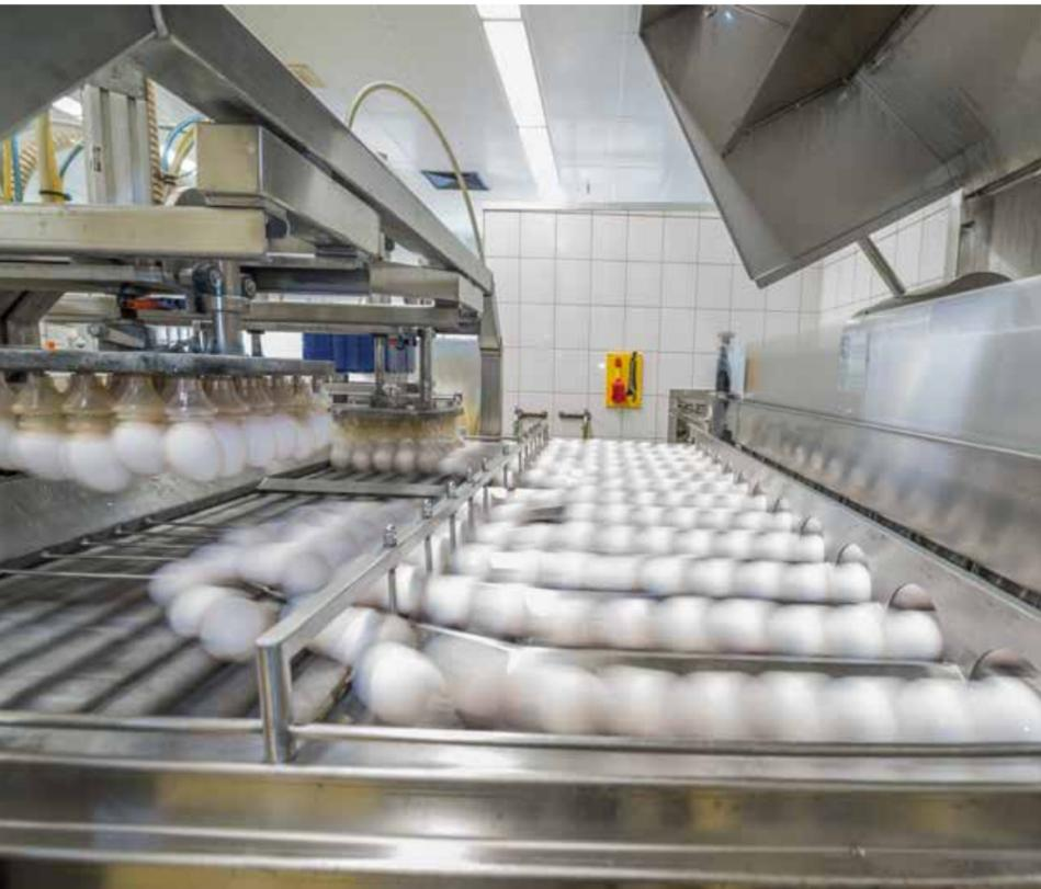
A purpose-made machine breaks the eggs and separates the yolks from the whites. Only the yolks are used in the process. The egg whites are sold on to other manufacturers. The machine can process 40.000 eggs per hour.
